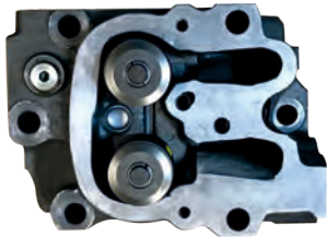
ÜRÜN ADI : SİLİNDİR KAPAĞI BOŞ PRODUCT NAME : CYLINDER HEAD (BLANK) ARAÇ ADI : MAN 19.422 VEHICLE ORJ. REF. NO : 51 031 016 585 ORJ. REF. NO ÜRÜN NO : C51031301 PRODUCT NO
